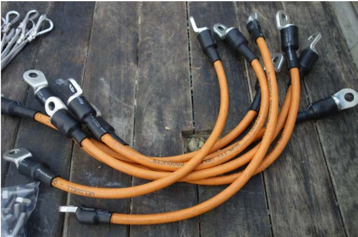
Figure 21: Electrical continuity bond cables
