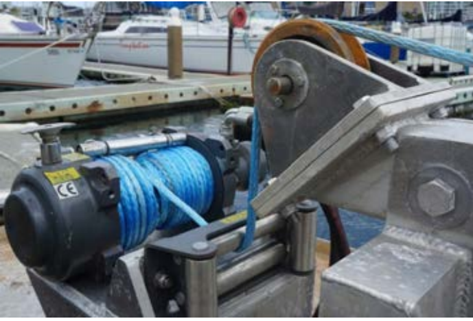
Figures 11 & 12: Load testing of mooring leg
