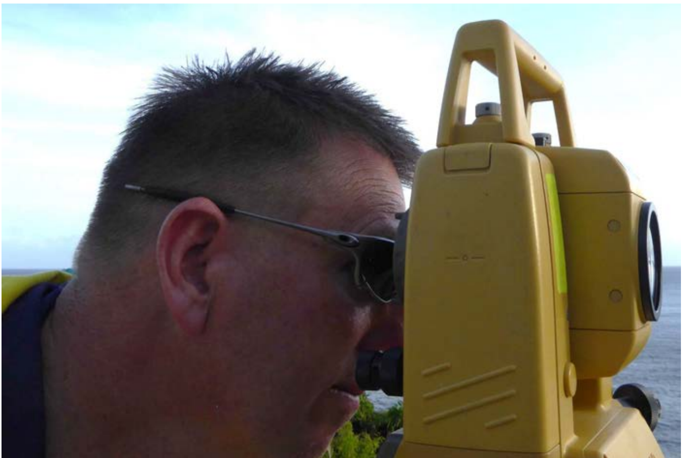
Figure 15: Monitoring 'Station' (Breakwater) movement under the influence of applied test loads
