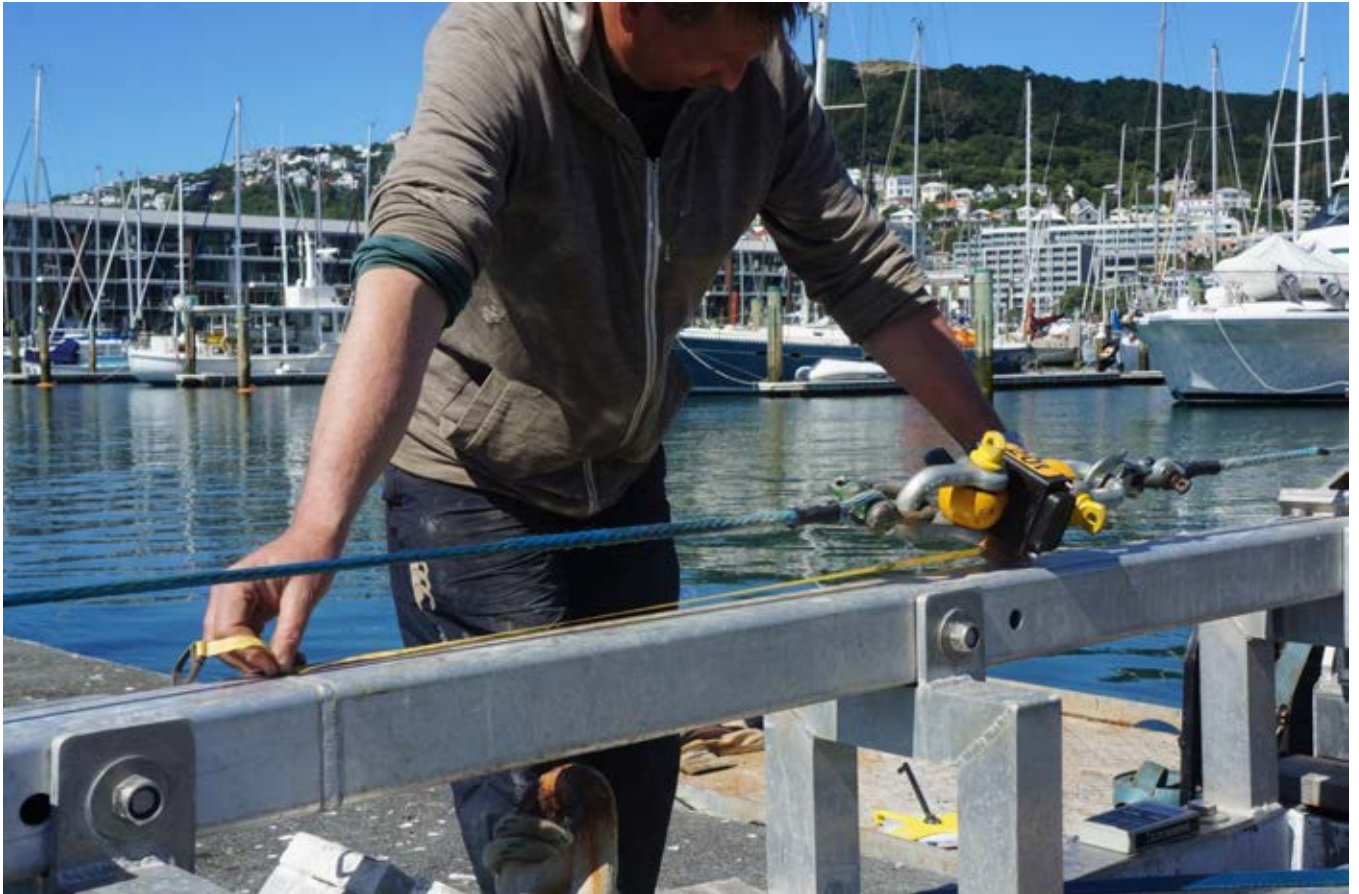
Figure 14 : The distance of travel checked with varying test loads being applied
