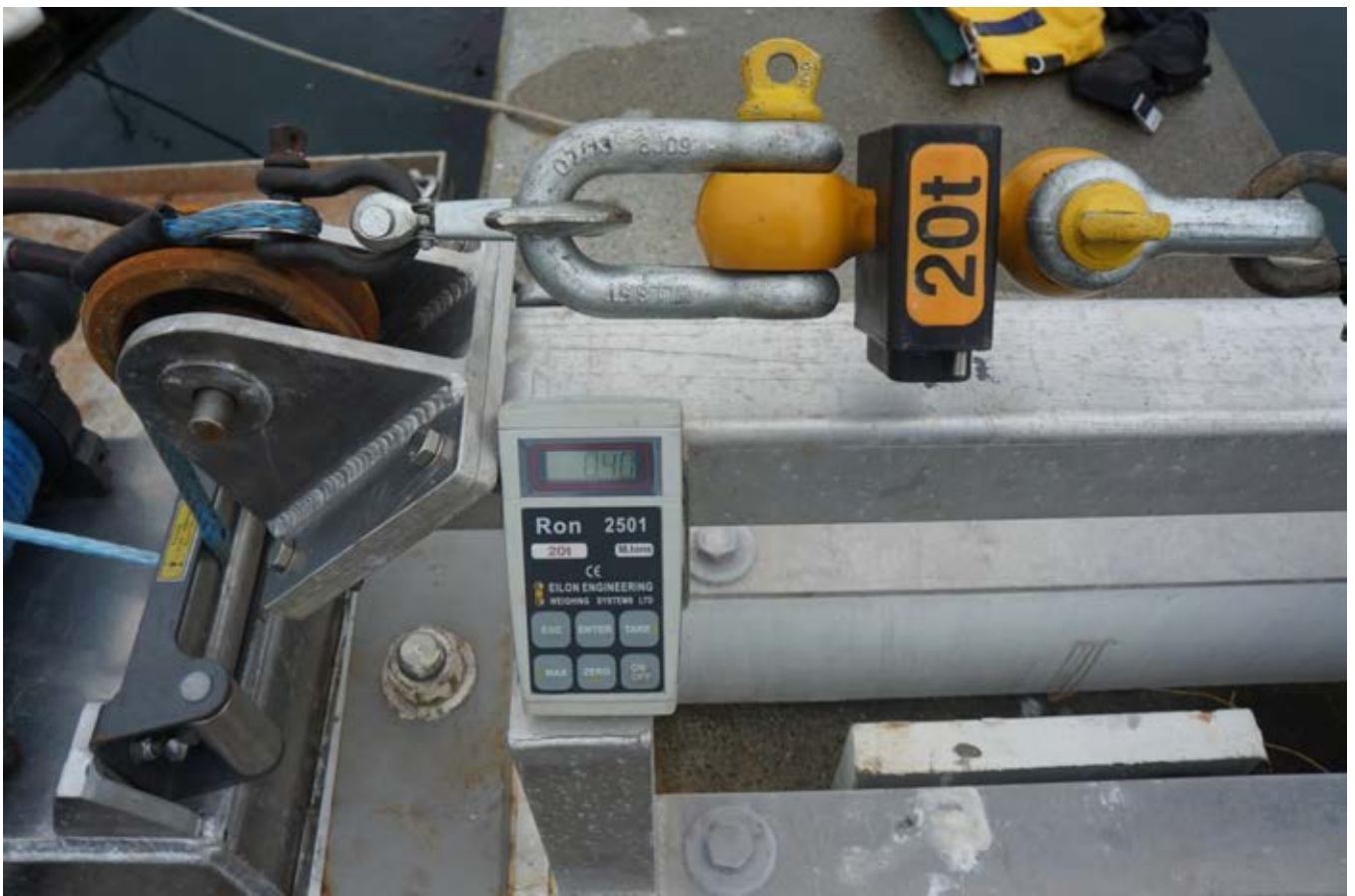
Figure 13: A pretension of 0.40 M.tons achieved the correct catenary angle on mooring chains Angle of chain at top connection to horizontal = 54^{\circ} (approximate: BW at rest, however tidal influenced) Angle of chain at top connection to vertical = 36^{\circ} (approximate: BW at rest, however tidal influenced)
