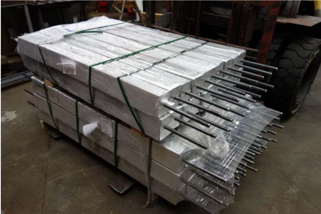
Figure 20: A50 (50kg ea.) sacrificial anodes
